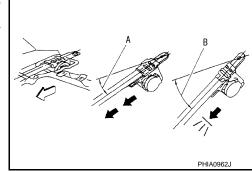
3. Replace the seat belt assembly if it does not operate normally.
