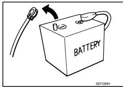
After installing the 12V battery, always check "Self Diagnosis Result" of all ECUs and erase DTC.
